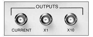
**X1 OUTPUT**: This BNC connector provides the measured signal (plus any DC offset) for recording on a chart recorder or oscilloscope.
