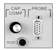
ring provides a coarse adjustment and the inner knob allows for fine control.
