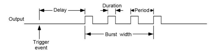
**DELAY:** These controls determine the time duration between the initiating trigger event and the beginning of the pulse burst. If this rate selector is set to **NONE** or the multiplier is set to **0.00** there is no delay.
