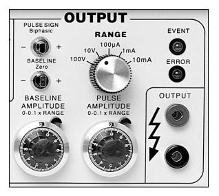
**RANGE**: This rotary switch determines if the output pulses will be constant current (3 ranges) or constant voltage (2 ranges).
