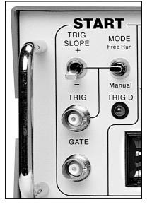
**TRIG**: This BNC connector allows a signal from an external source to initiate timing cycles. It is set for standard TTL levels.
