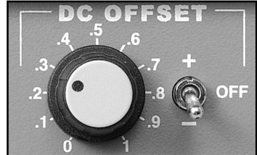
**DC OFFSET SWITCH (+ OFF -):** This switch sets the DC offset polarity or alternately turns the feature **OFF**.
