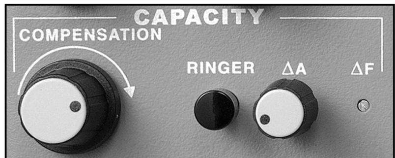
preparation using the internal squarewave generator and an oscilloscope connected to either the **X1 OUTPUT** or the **X10 OUTPUT**. This control should be adjusted to obtain the sharpest corners possible on the square-wave with very little overshoot. Clockwise rotation of this control increases the capacity compensation.
