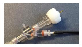
The outside of the Optopatcher should be wiped dry before insertion into the headstage. No electrolyte should be allowed to accumulate on the external surfaces and that no air spaces exist in the current path. To maximize Optopatcher life, it should be blown dry after use, wiped dry on external surfaces and stored without touching each other, in a dry atmosphere. Alcohol or other solvents are not suitable for cleaning. Use distilled water to soften and remove deposits.
