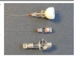
When shipped, the light fiber installed in the optopatcher is of considerable length; most likely it is longer than required for use. End users need to determine the final length they require based on their typical pipette length and trim the fiber accordingly. Optimum performance is obtained the closer the end of the light fiber is to the pipette end. Cutting the optical fiber to length is a simple task, provided you have access to an fiber optic scribe is used to score/snap the fiber.
