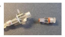
If replacing the fiber be sure to put the o-ring and gasket back on the fiber ferrule in the correct order.
