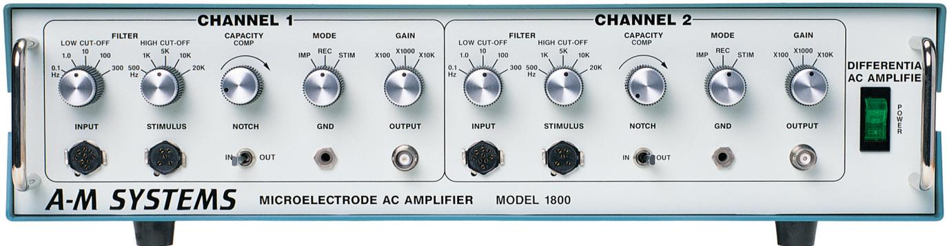
The Model 1800 AC Microelectrode Amplifier is a two-channel, differential amplifier configured for use with headstage probes. The instrument is intended for extracellular recording and/or stimulating in conjunction with high impedance metal microelectrodes. Ideal for single-cell spike recordings, it can also be used in a number of research or teaching applications requiring extracellular neurophysiological recording from excitable tissue such as nerve, muscle (EMG), EEG, EKG, and ERG recordings.
