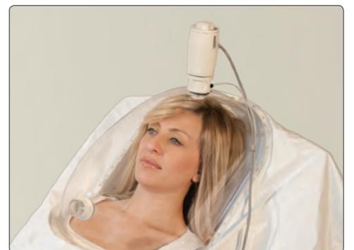
REE tests can be also performed (optionally) with a comfortable canopy hood
