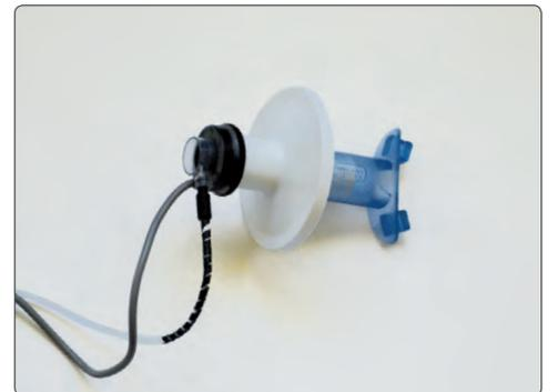
Ability to perform RMR test by using the "Mouthpiece & Nose-Clip" system
