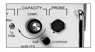
corners possible on the square-wave with very little overshoot. Clockwise rotation of both parts of this control increases the capacity compensation. The outer ring provides a coarse adjustment and the inner knob allows for fine control.
