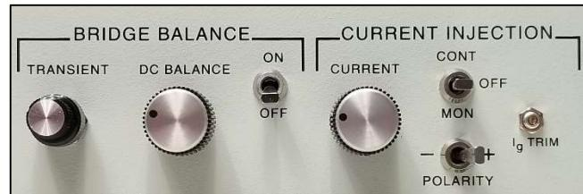
**DC BALANCE:** This knob controls a 10-turn potentiometer which nulls voltage drop across the electrode due to current injection when recording and stimulating through the same electrode. This function is disabled when the **ON\OFF** switch is set to the **OFF** position.
