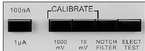
**1000 mV CALIBRATE:** This button provides an accurate reference signal for calibrating external recording instruments. It causes 1000 mV to appear at the **X1 OUTPUT** and 10 V at the **X10 OUTPUT**, in which case these two connectors are disconnected from other signal sources within the instrument.
