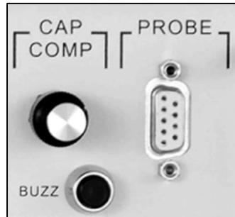
**BUZZ:** This button provides a capacitance override to send the circuit into positive feedback and cause the electrode to vibrate. This is commonly called a "tickler." When the electrode vibrates rapidly it sometimes will aid in the penetration of the cell membrane, or clearing of a clogged electrode.
