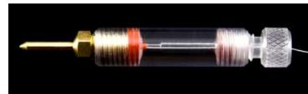
If the micropipette must have freedom of movement or "float," as when recording from moving muscle fibers, place the end of a thin chloride silver wire into the stem of a filled micropipette, securing the wire at the open end of the pipette with a fast drying cement. Solder the other end of the wire to a 2.0 mm diameter pin connector (Catalog # 521000). Coil the wire between the pipette and pin connector into spring. Insert the clean and dry pin connector in the Headstage.
