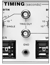
**TRIG OUT (LOWER):** This BNC connector provides a signal which is coincident with the Duration timing signal which controls pulse output.
