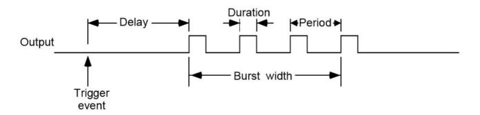
**DELAY:** These controls determine the time duration between the initiating trigger event and the beginning of the pulse burst. If this rate selector is set to **NONE** or the multiplier is set to **0.00** there is no delay.
