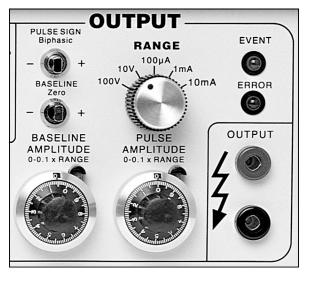
**BASELINE AMPLITUDE:** This value is independently set using a ten-turn counting dial. The maximum baseline amplitude is one tenth the value shown on the range amplitude switch
