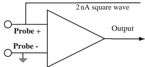
The current source consists of several parts. A square wave is applied to an active current source, which converts the square wave voltage to a square wave current of 2nA p-p at 100 Hz. The calibrated current source is connected to the electrode leads.
