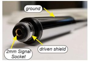
particularly sensitive to stray electric fields, due to the high impedance of the electrode tip and the Headstage input. Using a driven shield for this purpose has the advantage of not introducing any additional shunt capacitance nor a path for current leakage to ground.
