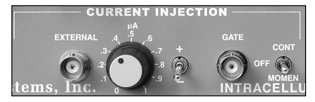
**EXTERNAL**: This BNC connector provides control over the magnitude of the injected current via an external signal applied at this input. The current applied here is summed with the current set by the **µA** knob. Sensitivity is 100 nA/V. Current injection is triggered via the **CURRENT INJECTION (CONT-OFF-MOMEN)** switch or the **CURRENT GATE** connector.
