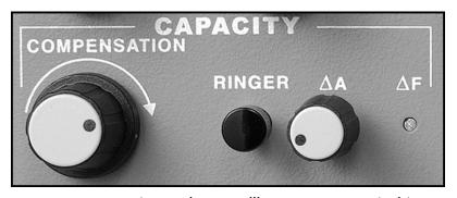
preparation using the internal squarewave generator and an oscilloscope connected to either the **X1 OUTPUT** or the **X10 OUTPUT**. This control should be adjusted to obtain the sharpest corners possible on the square-wave with very little overshoot. Clockwise rotation of this control increases the capacity compensation.
