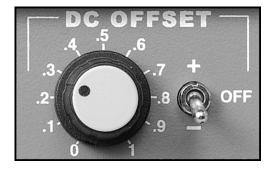
**DC OFFSET SWITCH (+ OFF -):** This switch sets the DC offset polarity or alternately turns the feature **OFF**.
