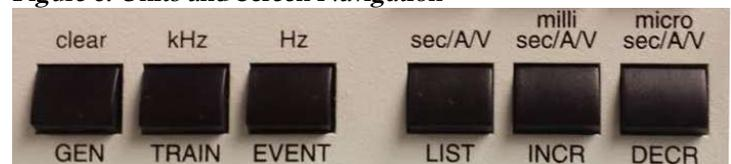
SEC/A/V sets the units to Seconds or Amps or Volts as appropriate for the active variable.
