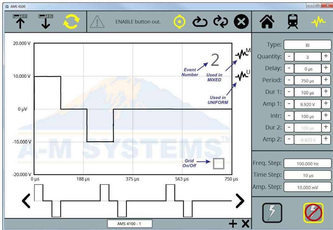
Event parameters can be entered in the right hand column. Amplitude and Durations can be adjusted by clicking and dragging (or using touch screen gestures) on the middle graph of the waveform.
