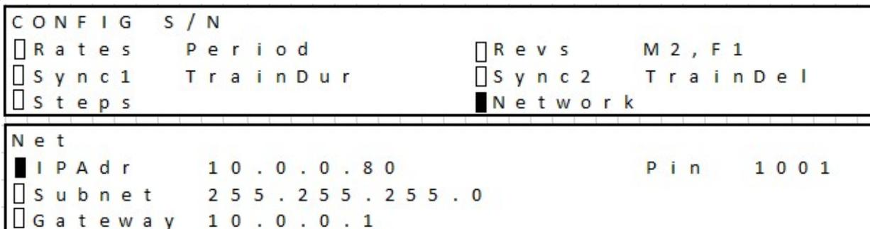
Navigate to IP Address and set the values to an approved number on your network. For this example, the Model 4100 will be assigned “10.0.0.80.” Note that it is unlikely that the Subnet and the Gateway numbers require attention. A PIN (can be user modified) is used to prevent unauthorized access to the unit via software. This number must also be entered into the software application in order for the software to control the instrument.
