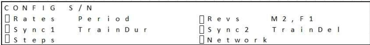
**RATES** determines if timing variables are entered in units of *Period* (microseconds, milliseconds, or seconds) or *Freq* (Hz, kHz).
