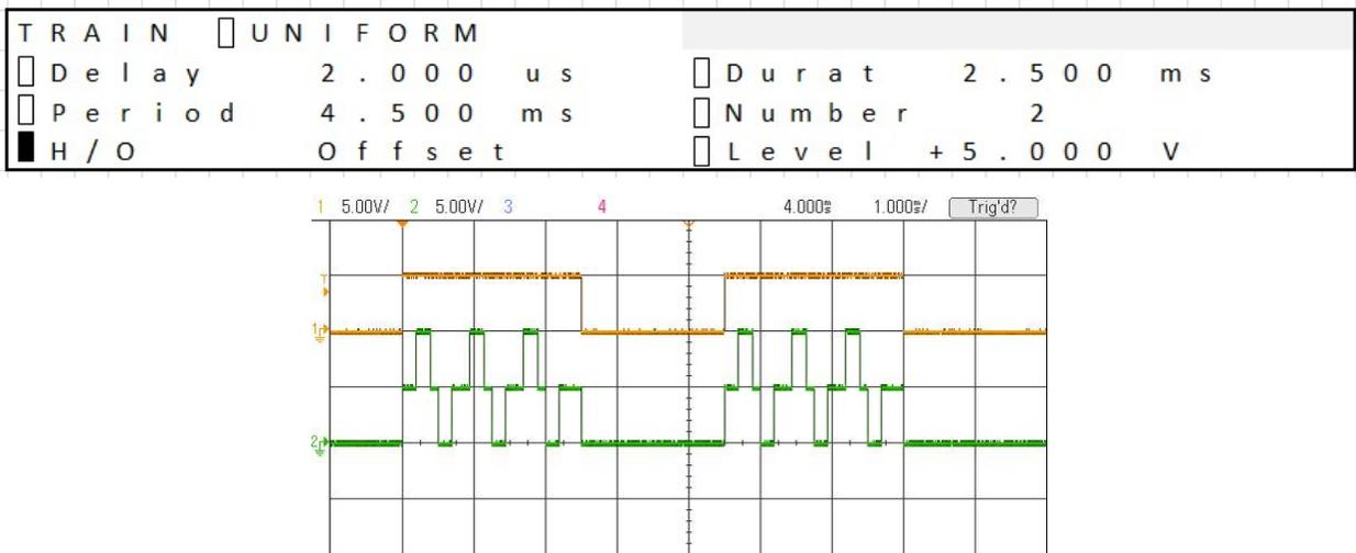
Also note that the amplitude of the biphasic pulse is determined using the **OFFSET** value as the baseline, so in Figure 70, it is a +/- 5V change from an offset of 5V, meaning the amplitudes end up at +10V and 0V respectively.
