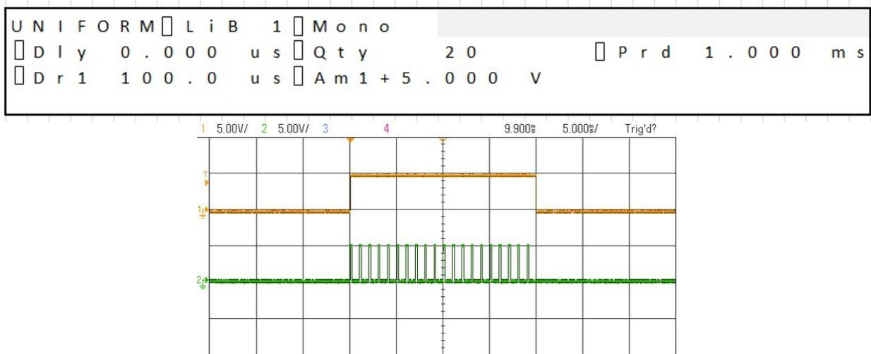
➔51. Change **GEN**. Set AUTO to *None*. Change your oscilloscope timebase to *1ms/div*.
