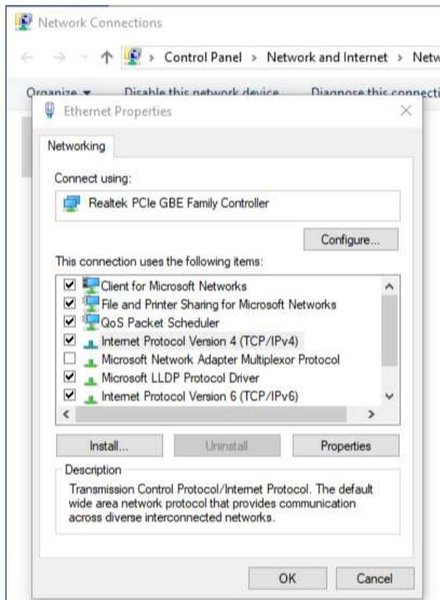
Enter an IP address that is nearby the value you want to set the Model 4100 address to. In this case, the computer network card was set to 10.0.0.81.
