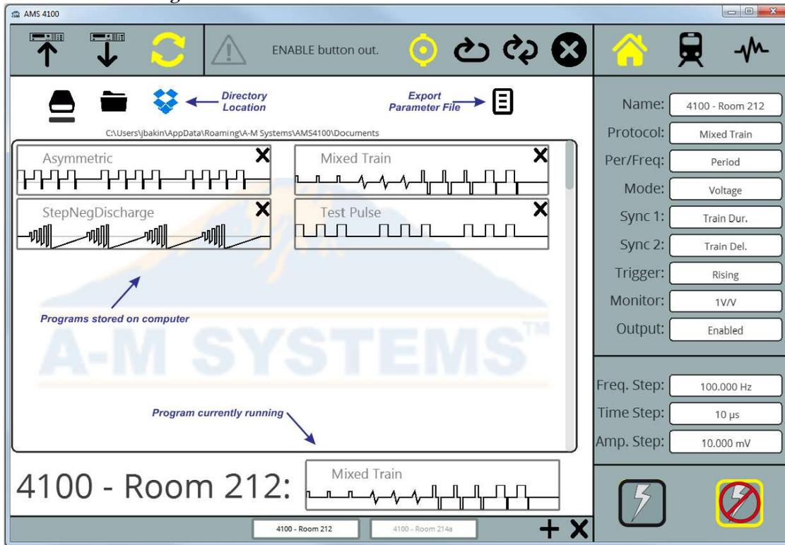
An additional feature that the software provides that is not present on the instrument itself is the ability to store multiple programs of stimulus information, and quickly change between programs. Programs are stored by dragging the current formulation up to one of the eight program slots. Programs can be uniquely named while in the Current position by clicking within ID box in the upper right.
