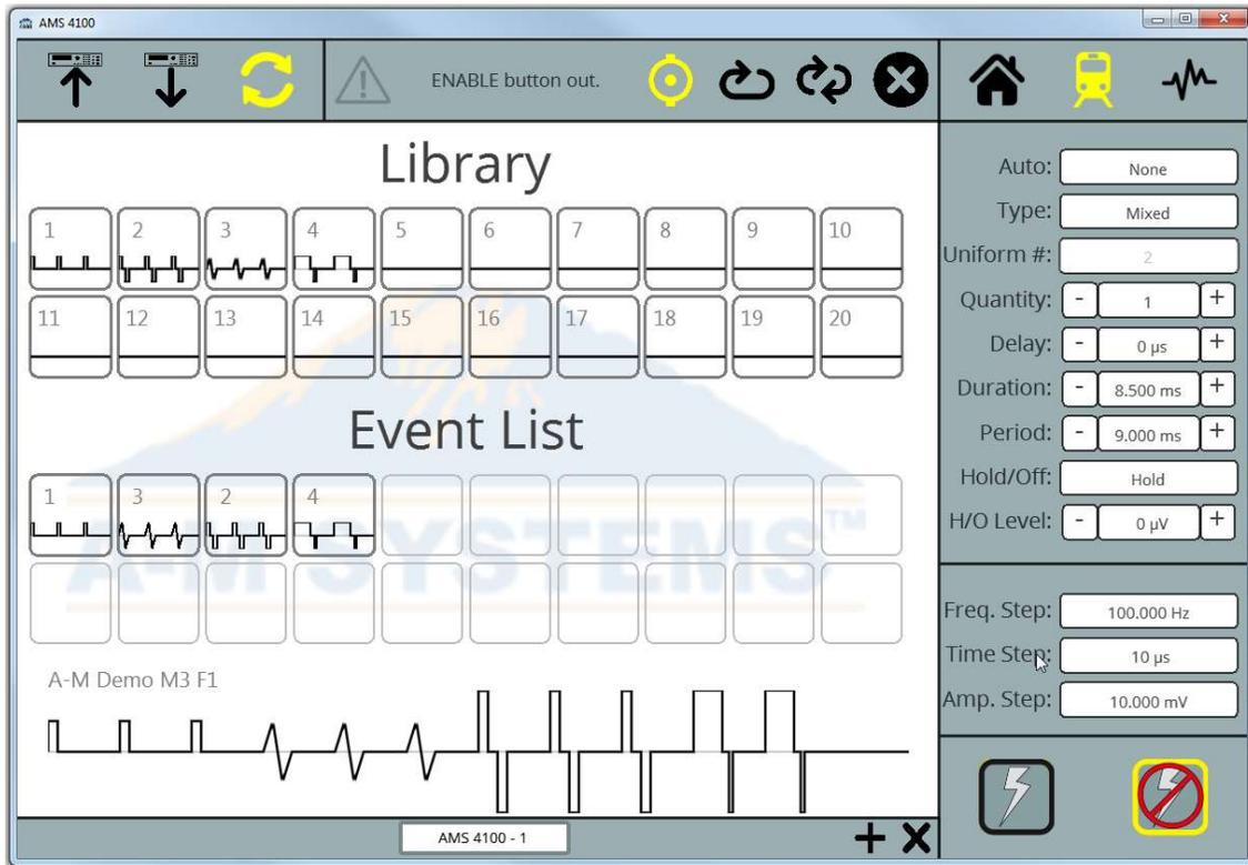
Events in the library can be dragged down into the Event List to set up the order in which they are delivered. Rearranging the event icons immediately results in reordering the events being generated by the 4100. Pulling an event icon off the Event List removes that event from the ones being generated.
