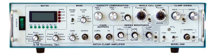
The Model 2400 Patch Clamp Amplifier is a low noise, full featured patch clamp designed for voltage clamping using patch electrodes on single channels or whole cells. Amplifier current gain can be matched to your experimental needs by selecting one of the three available dual resistive feedback probes. Currents with outputs of 10mV/nA to 1mV/fA can be recorded. *(See Specifications on the reverse side for details).*
